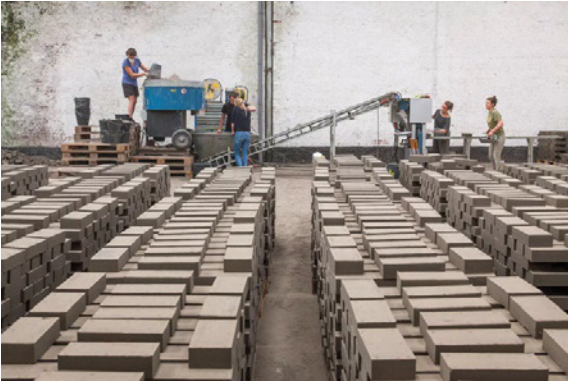
Figure 5. Fort V, Regional house of the Edeghehem commune, BC Architects. Volunteers help to work on the production of more than 19,000 compressed earth blocks using locally sourced clay. Photo credit Thomas Noceto
